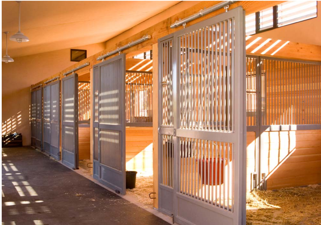
NATURAL LIGHT FILLS THE STALL AREA. STALL FRONTS, DOORS AND PARTITIONS ARE POWDER COATED STEEL. THEY WERE CUSTOM MANUFACTURED IN KENTUCKY.
